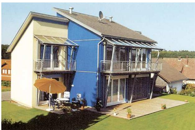
Example of a typical self-sufficient “Zero Energy” house in Germany featuring a combination of active and passive solar energy and space heating by biomass.
